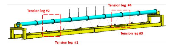
Fig. 1 Geometry of submerged floating tunnel
